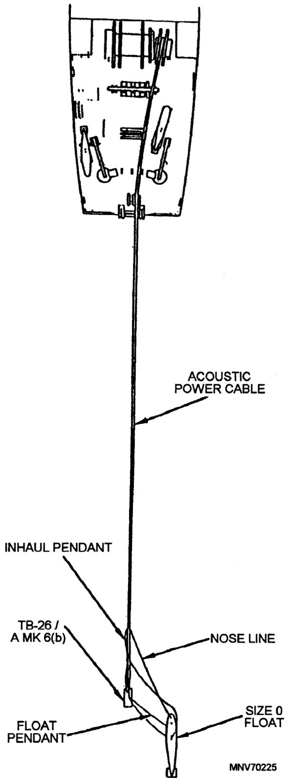
Figure 9-8.—Acoustic sweep configuration TB-26/A Mk 6(b) astern.
